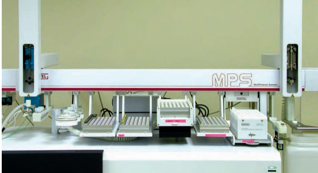
MultiPurpose Sampler (MPS XL) with GERSTEL DPX Option used for the automated hydrolysis and DPX-LC/MS/MS method shown mounted on top of an Agilent 6460 LC-MS/MS system without adding to the lab bench footprint.
