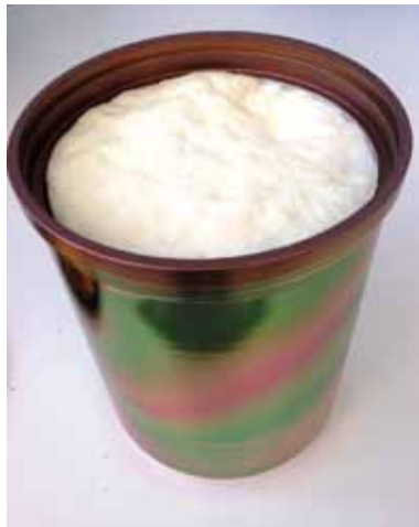
The cutting tool remains in place and surrounds the sample throughout the analysis, meaning emissions escape and can be measured exclusively via the surface that is typically in contact with the surrounding air.
