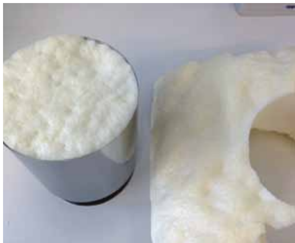
The PU sample is taken using a special cutting tool, which is also used as sample holder.
