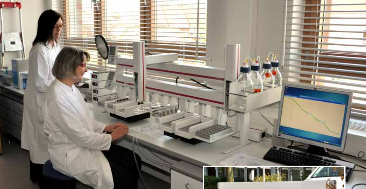
MPS PrepStation in the LAVES laboratories. Due to its "wing span", the staff refers to it as "Condor". The MPS guarantees uniform results when generating standard solutions even when operated by different users.
