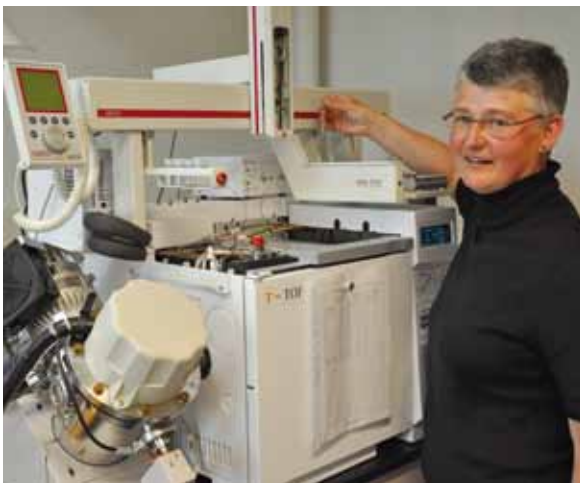
GC/TOF-MS for pesticide screening: Thanks to the GERSTEL MPS with Automated Liner Exchange (ALEX), even series of “dirty” samples are easy to analyze.
